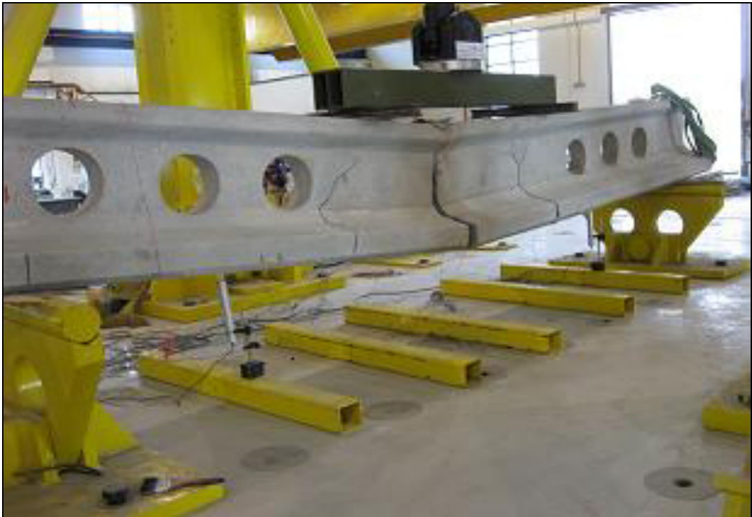
Figure 8. Flexural failure of beam with 3 web openings in constant shear area
