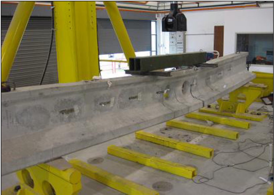
Figure 12. Flexural failure of beam with 2 web openings in constant moment area
