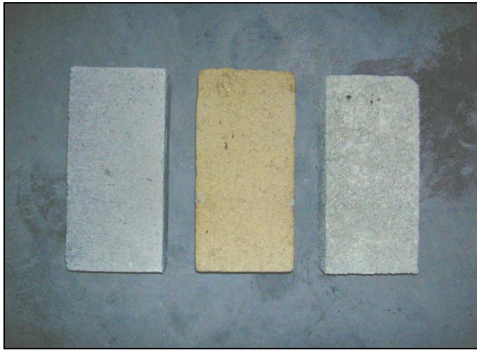
Figure 1. Brickwork unit used in the investigation (Calcium silicate-left, clay brick-centre, cement sand brick-right)
