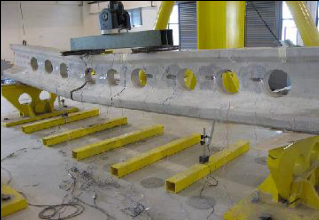
Figure 6. Flexural failure of beam with 9 circular web openings
