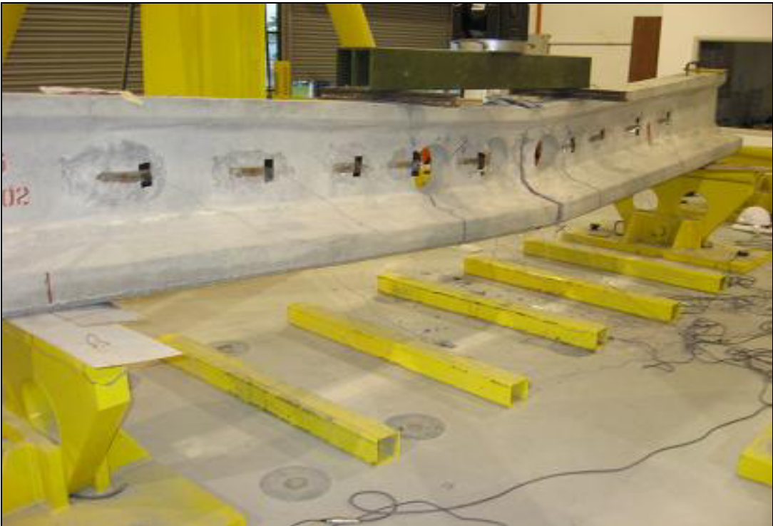
Figure 10. Flexural failure of beam with 3 web openings in constant moment area
