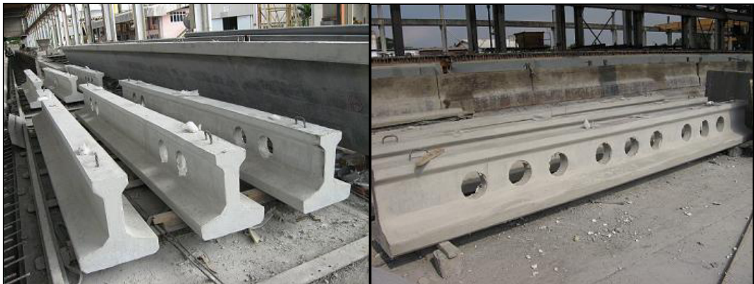
Figure 4. Pretensioned Inverted T beams with circular web openings fabricated at Hume factory
