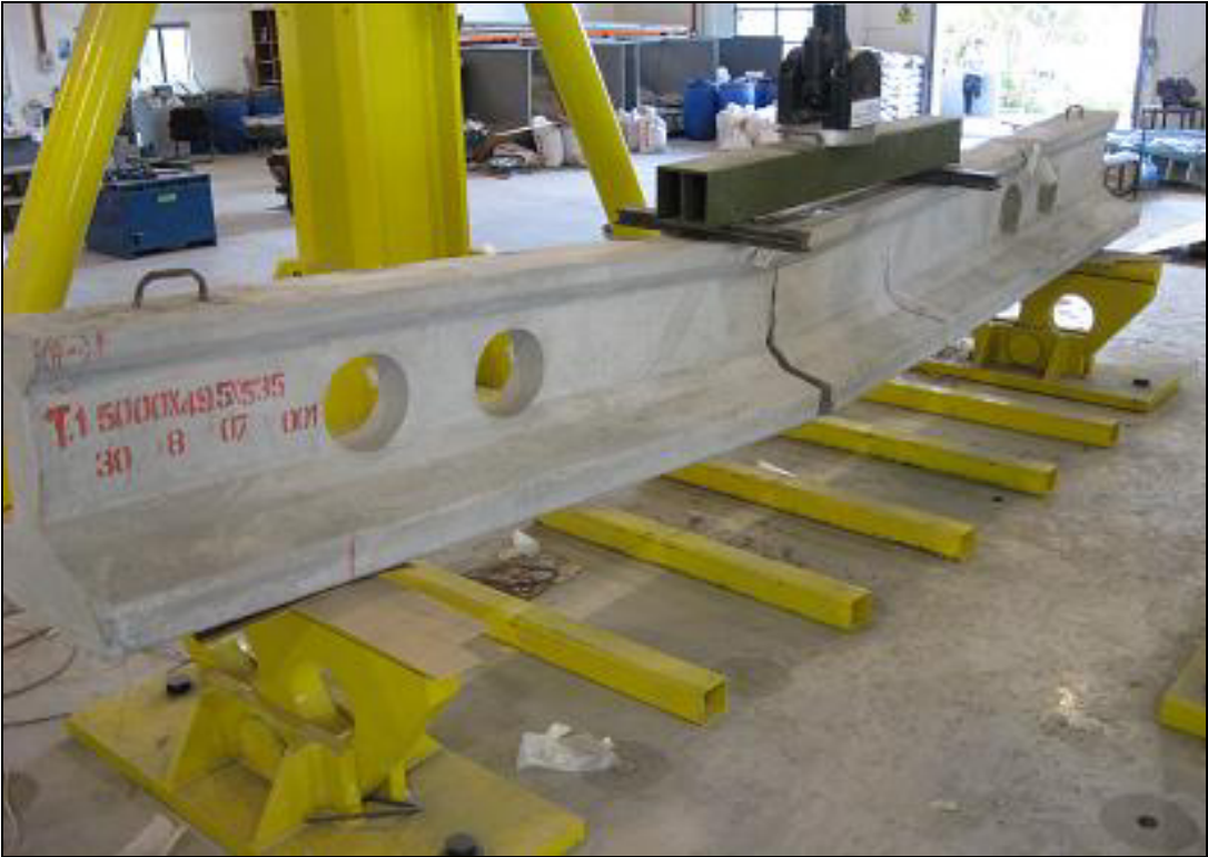
Figure 14. Flexural failure of beam with 2 web openings in constant shear area
